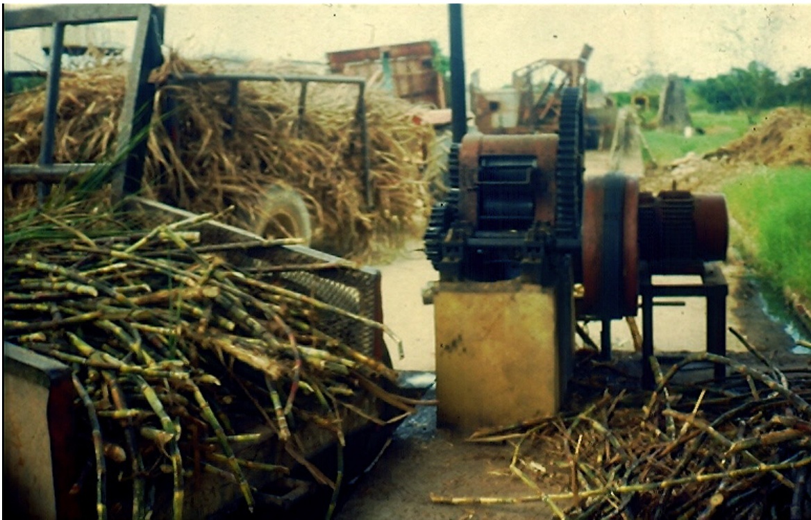
Figure 7: Sugarcane roller juicer at the SFC, Trinidad
