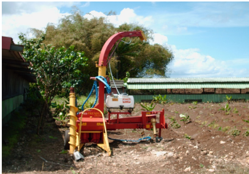
Figure 6: Forage harvester used for harvesting and chopping standing sugarcane and erect type forages.
