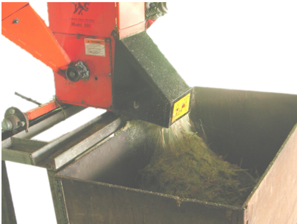
Figure 21: A stationary chopper for processing small quantities of sugarcane.
